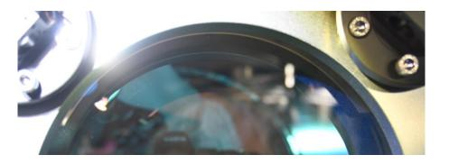
The center area looks clean. But there is FC residue on its lower right side. And it still has dirt on its upper side and a lot of dust on its lower right that couldn't be found in this picture. Because these are on the out-of-jig range, we couldn't do anything more.
